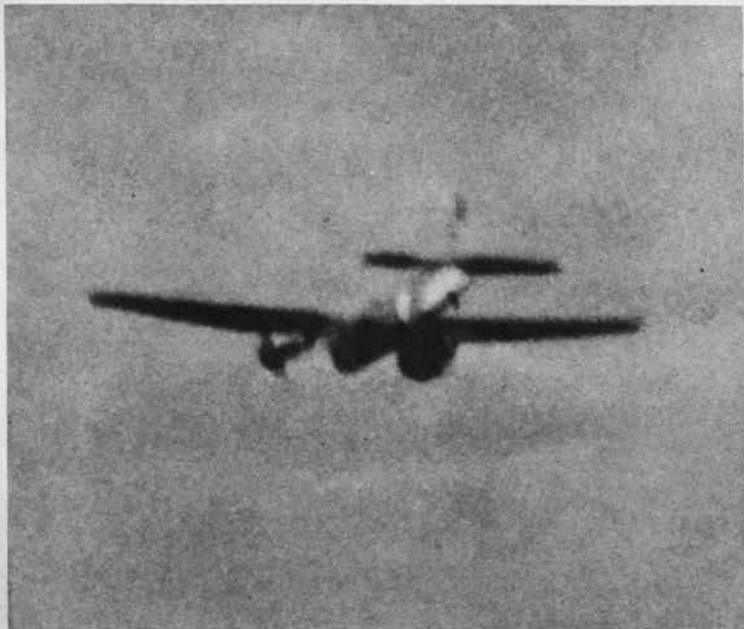
Frances' tail comes to a point, thus distinguishing the plane from Irving whose tail tapers gently. Its wingspan has only slight dihedral.
